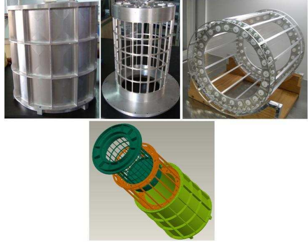
Fig. 4. Fabricated parts of the cylindrical detector and the total assembly
