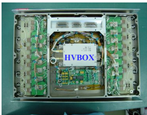
Fig.9. Back side of the PC. Electrical circuits are mounted. Seven readouts are connected to the left and right preamp boards. The low-power high-voltage box is in the middle.
