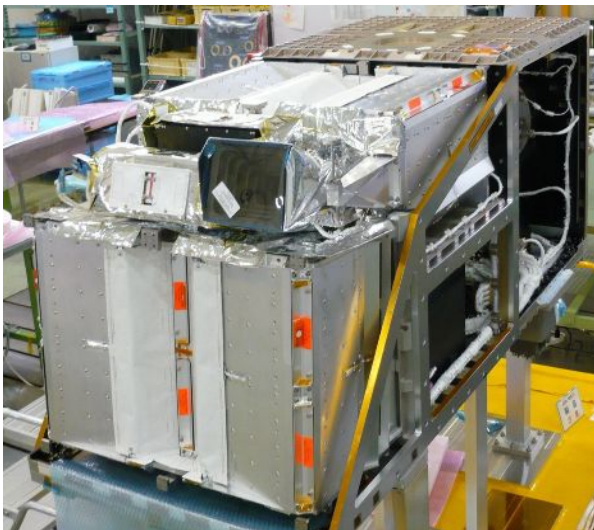
Fig.5. MAXI in the electric test. Six cameras in forward direction are facing us. The middle two cameras in the center are hidden. See also Fig.2.
