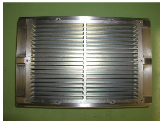
Fig.7. Proportional counter used in GSC. The body size is 358 \times 236 mm. The Be window is 100 \mu\text{m} thick and He-leak tight.
