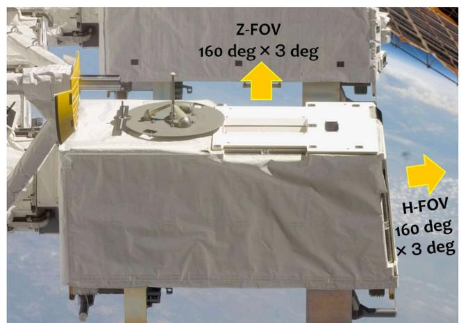
Figure 1. Real MAXI on ISS. Photo taken from the docked space shuttle (©NASA). Right-hand side is the moving direction of ISS. MAXI has two FOVs.
