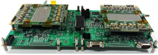
Fig. 2. A picture of the sensor boards stacking on the readout boards of the T-LEX prototype model.
